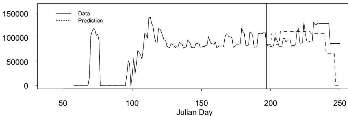
Figure E-8 Spill predictions and observations for Bonneville Dam. Y axis shows CFS.
