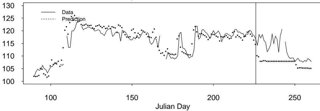
**Figure I-4** Total Dissolved Gas predictions and observations for Priest Rapids Dam as measured at PRXW. Y axis is the percent saturation.
