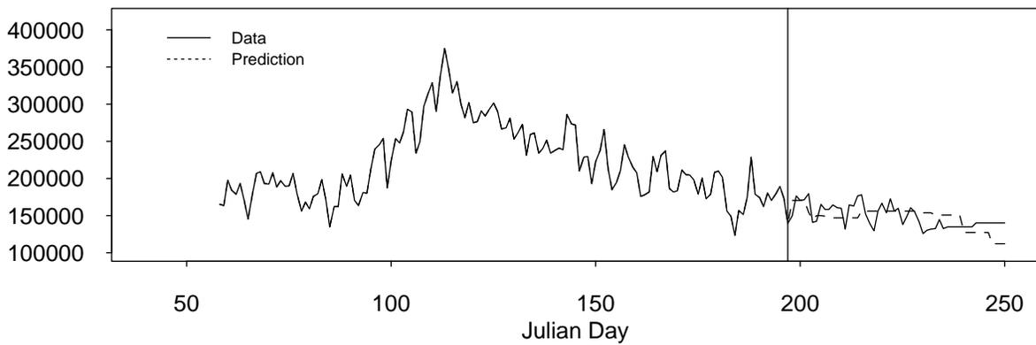
**Figure E-5** Flow predictions and observations for The Dalles Dam. Y axis shows CFS.
