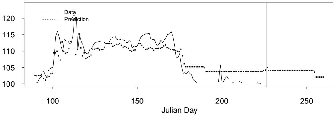
**Figure I-2** Total Dissolved Gas predictions and observations for Little Goose Dam as measured at LGSW. Y axis is the percent saturation.
