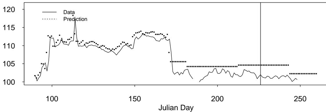
**Figure I-1** Total Dissolved Gas predictions and observations for Lower Granite Dam as measured at LGNW. Y axis is the percent saturation.
