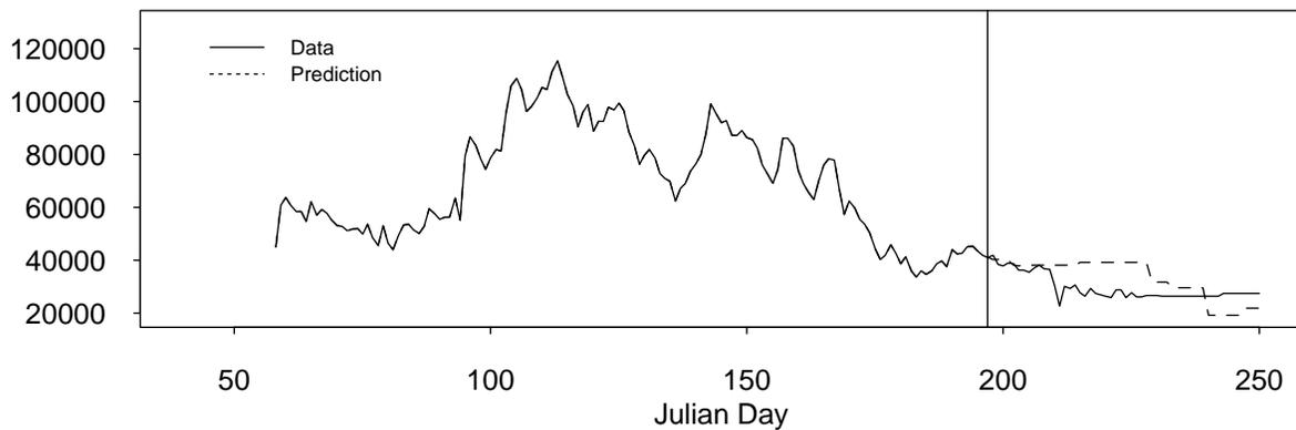
**Figure E-1** Flow predictions and observations for Lower Granite Dam. Y axis shows CFS.
