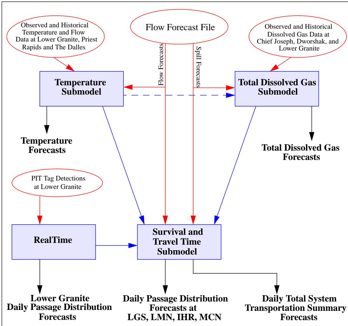
**Figure 1** Simplified schematic of RealTime and CRiSP complex. Prior to migration year 2000, model generated gas was not updated with observed values for the production of daily passage distribution forecasts. PIT Tag data courtesy of Pacific States Marine Fisheries Commission. Water Quality Data courtesy U.S. Army Corps of Engineers. Flow Forecast File provided by Bonneville Power Administration and U.S. Army Corps of Engineers.
